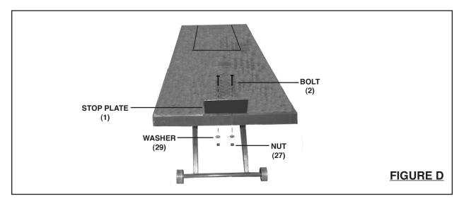
2. Align the two mounting slots in the Stop Plate (1) with the two mounting holes located at the rear of the Platform (8). Then secure the Stop Plate to the Platform, using two Bolts (2), two Washers (29), and two Nuts (27). **NOTE:** When adjusting the Stop Plate forward or backward, make sure to retighten the two Nuts. (See Figure D.)
